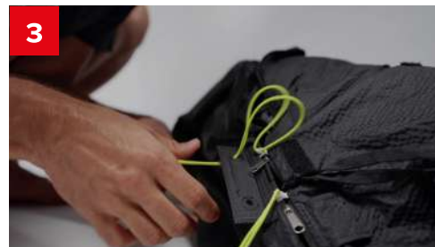
3 Place the Rescue Handle in place through Velcro. Keep plastic wires through both white straps
