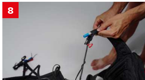
8 Anchor the tube in the resting position
